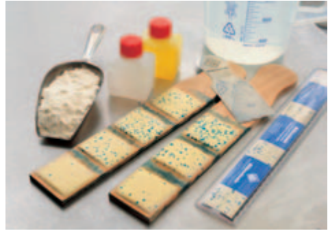
Fig. 108: Wet Pekar sample with Tauber's reagent for determination of ascorbic acid
